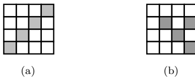
Figure 3: Illustration of Zero Difference Pattern (ZDP) for an AES state. The gray colored bytes denotes the active ones, whereas the white ones denote the inactive bytes. In this case, if each diagonal is considered as a word, then the ZDP of Fig. 3a and Fig. 3b are (1, 0, 1, 0) and (0, 1, 0, 1) respectively; whereas if inverse diagonals are considered as a word, then the ZDP becomes (1, 1, 1, 0) and (0, 1, 0, 1) . Note that, the diagonal (inverse diagonal) containing the i -th byte ( 0 \leq i \leq 3 ) of the first row is considered as i -th diagonal (inverse diagonal).
