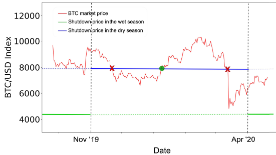
Fig. 4: An example of mining machine switch mechanism considering wet-dry season transition. The red line represents the BTC market price in USD. The green line represents Antminer T9+ shutdown price with low electricity fees in the wet season, while the blue line represents the shutdown price with high electricity fees in the dry season. The red X represents the shutdown point for this mining machine, when BTC price decreases and triggers that point, the machine should be switched off, while the green circle represents the re-open point, when the BTC price hits the point upward, the machine should be switched on.
