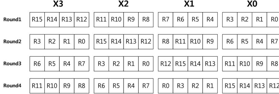
**Fig. 1.** Register alignments for LEA encryption in AVR
