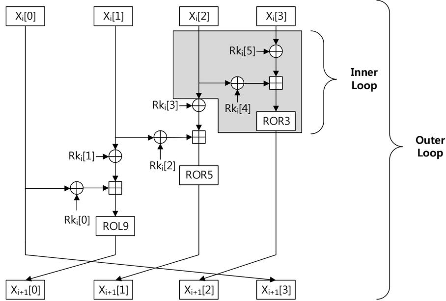
**Fig. 2.** Inner and outer loops of LEA encryption
