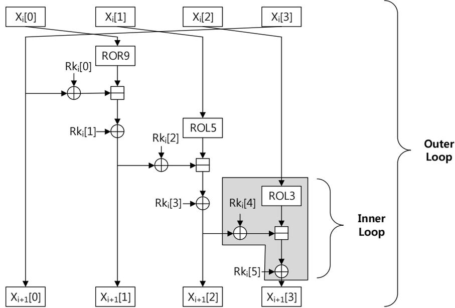
Fig. 3. Inner and outer loops of LEA decryption
