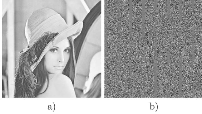
Fig. 3. The encryption result when  $K = \text{"3C1DE8FF0151FF012840"}$  (represented in hexadecimal format, the same hereinafter): a) the red channel of the plain-image "Lenna"; b) the red channel of the cipher-image. For the other two color channels we have obtained similar results.
