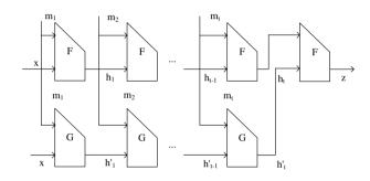
Fig. 6. The Improved Double-Pipe Hash
