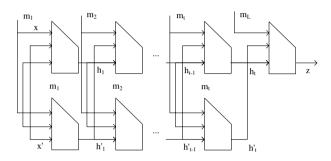
Fig. 3. The Double-Pipe Hash
